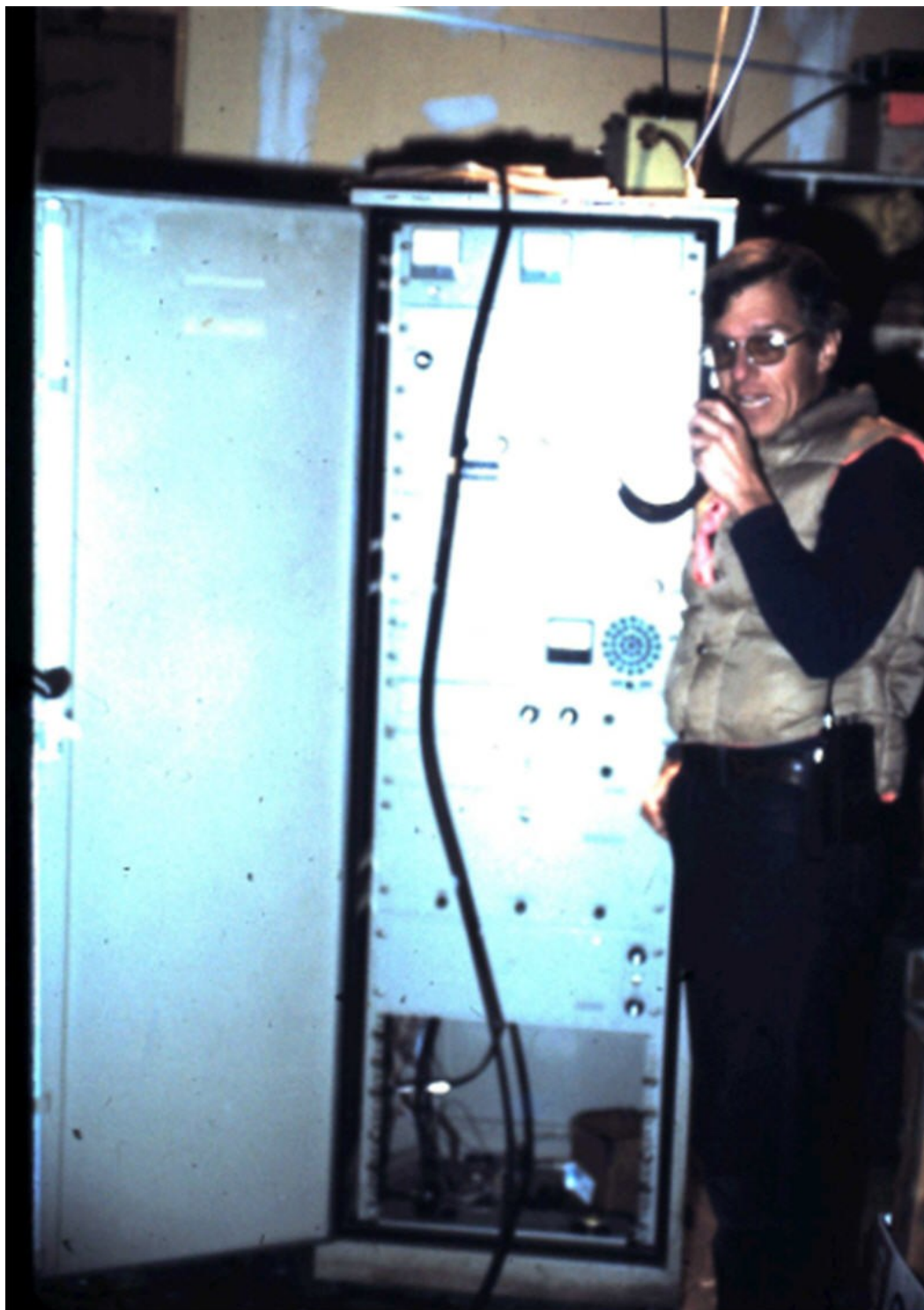
Fall, 1983 - Testing the DRC Motorola Motrac 147.33 repeater / Dave, wg0n
