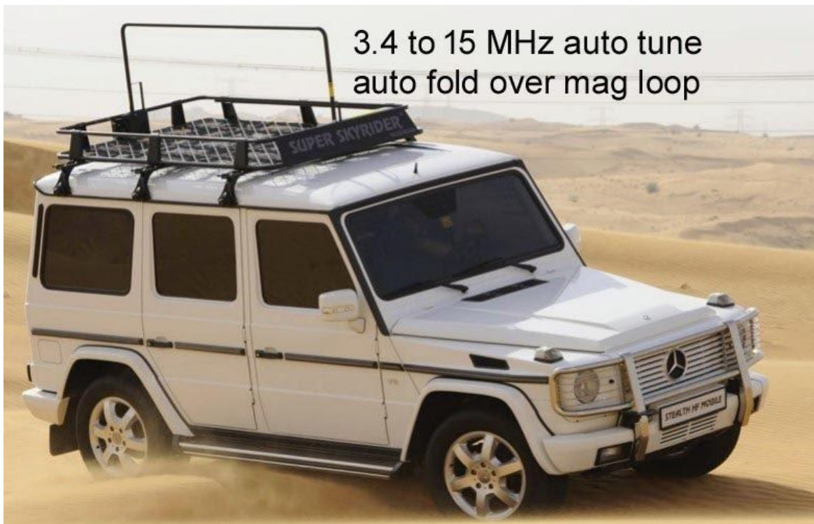
Figure 7 - Commercial NVIS loop antenna made by Stealth Telcom
