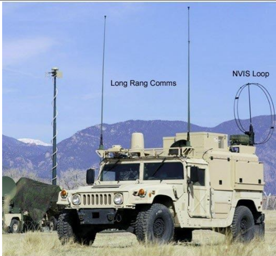
Figure 6 - Military command vehicle equipped with NVIS and long range comms
