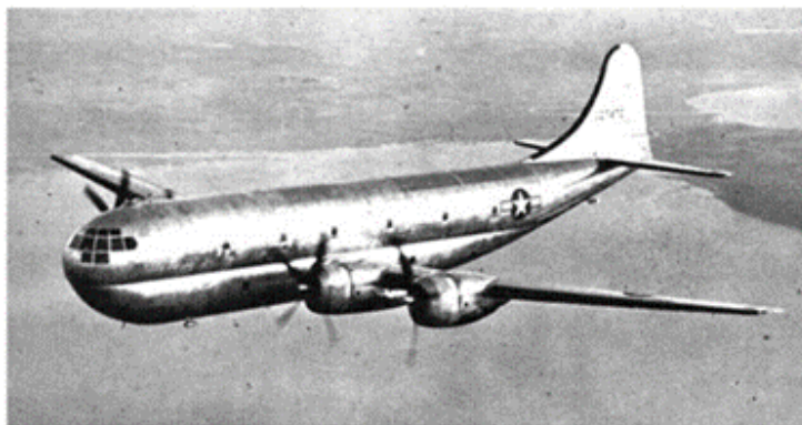
The C-97 is a military cargo version of the Boeing Model 377 Stratocruiser, super-airliner.
