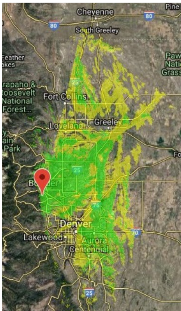
W0BTV - DATV Repeater Coverage Area Green shaded areas are strong signals. Yellow shaded areas are weak signals of less than 10dB above digital threshold.
