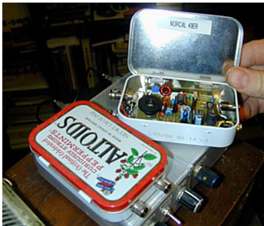
Figure 1 - 1.2 watt homebrew 40 meter CW transceiver
