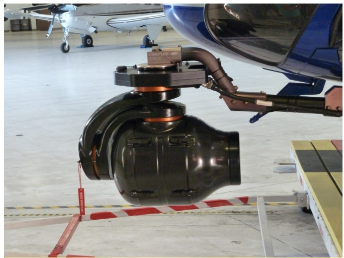
Retracted Chopper Camera
