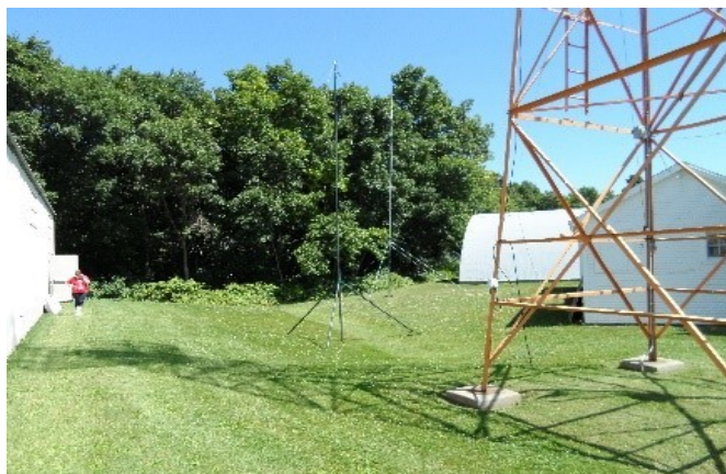
W9ZL Special Event Station antennas. A dipole, a trap vertical, and a six meter Discone.
