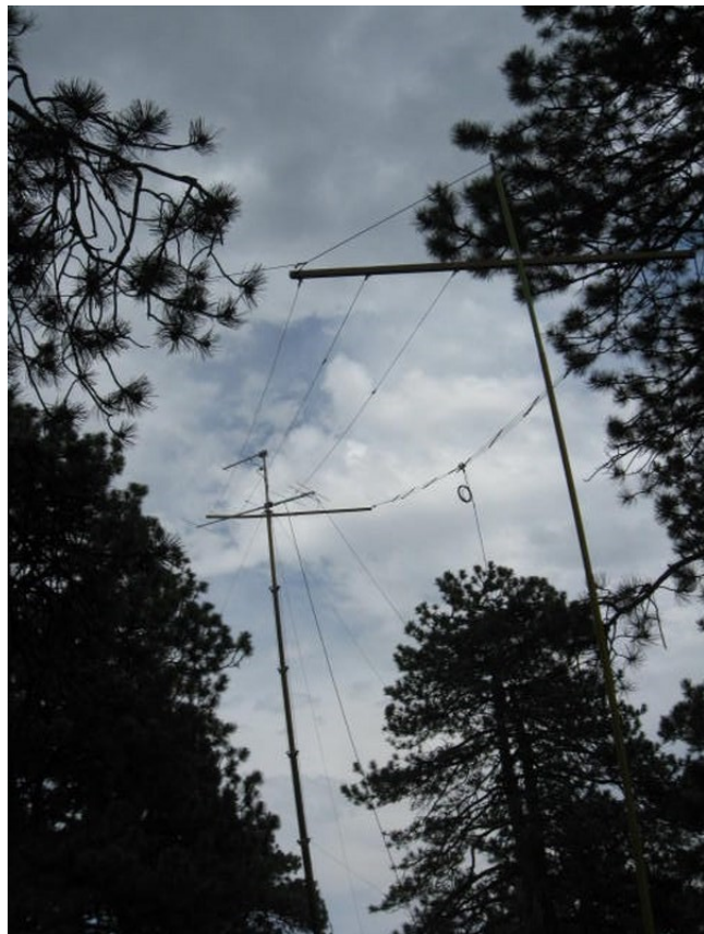
The wire beam's up, supported by a pump up mast at one end
