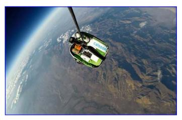
Inside the payload, there was a high-energy radiation sensor, a cryogenic thermometer, multiple GPS altimeters and trackers, and three cameras. During the 2.5 hour flight, the buoy collected more than 50 gigabytes of video and science data ranging in altitude from 8500 ft to 113,700 ft above sea level. The analysis is still underway.
