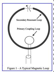
Figure 1 shows the configuration of a typical magnetic loop antenna. Magnetic loops have been very popular for years in many countries and are becoming very popular in the United States. The reason is because more hams are moving to covenant controlled areas which do not allow antennas or into condos or townhomes where installing outside antennas is an issue.
