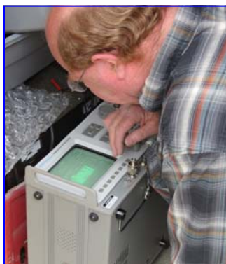
Paul is using a Service Monitor to check signal levels.
