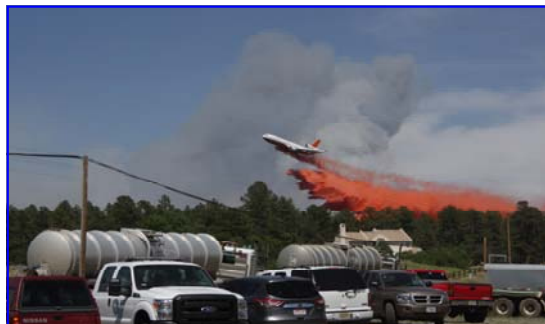
A DC-10, VLAT (Very Large Air Tanker) drops 11,000 gallons of fire retardant on the Black Forest Fire at Colorado Springs in June 2013. Photo - Dave Baysinger
