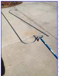
First I bought two 10 foot lengths of 3/4" EMT conduit (\$4 ea) because I already had a bender in my toolbox. Bending the hook was easy. I made three hooks and bolted them together with 10-24 hardware. A piece of 1" dia PVC pipe is used as the insulator at the base to keep the EMT from touching the radial plate. I borrowed a couple of genuine feeders from my wife as
