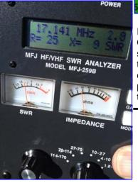
ence. A dip at 29MHz would have been consistent with what I have researched. Seventeen MHz means the antenna has an electrical length of 13 feet. Suspicious but I guess the proof would be if it gets out like a 13 foot antenna.
