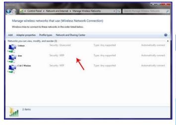
**Step 3** - Deselect "Connect automatically when this network is in range". Click "OK". Repeat steps 2 and 3 for any other network set for auto connect (except for "trusted networks" such as your home network).
