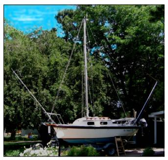
I was able to solve the SWR problem by extending the legs from the bow and the stern using a 14-foot telescoping boat hook and a 14-foot whisker pole. Both of these sailing items I already had on the boat. Using these extensions, I got an angle between the legs of about 145 degrees, and the SWR dropped down into the range of 1 - 1.3 in the 20 meter band frequencies. The SWR and impedances that I got once the boat was on the water at Granby were as follows:
