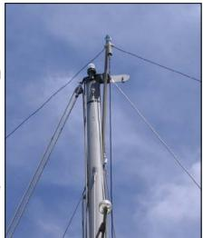
Prior to taking my boat to Granby, I staged it in my driveway, erected the mast, and tried out the inverted V with one leg going from above the top of the mast to the bow, and the other leg to the stern. This antenna configuration resulted in SWR well over 3 in the frequencies of the 20 meter band. The angle between the legs of the inverted V was only about 6 5 degrees, and the legs were quite close to some of the metal standing rigging of the boat. (*See Photo on Page 4*)
