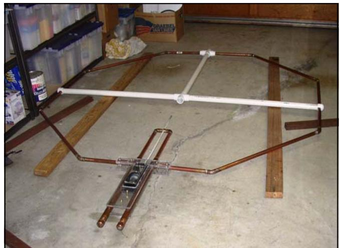
Starting at the capacitor each of the octagon sections were soldered in turn. I first had the control wire through the sections of the loop but after soldering the first few sections I found that the control wire had melted. So I used it to pull a stainless steel wire through the original sections and the remaining unsoldered sections and then pulled a new control wire through the loop after all of the soldering was done.
